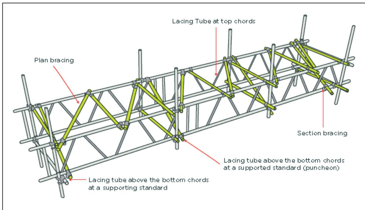
A pair of trusses acting as a bridge between two pairs of supporting standards
