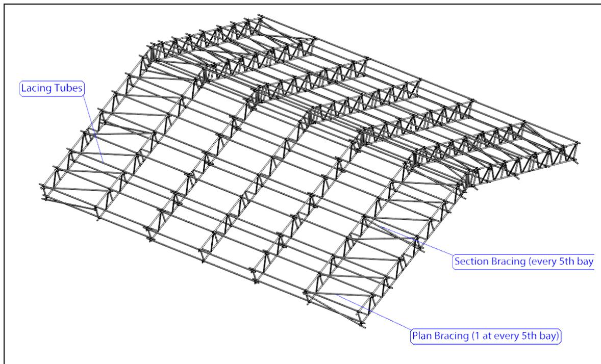
Double pitched roof utilising trusses as rafters.
